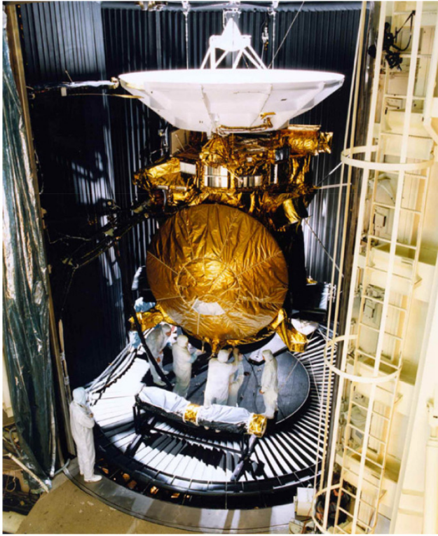
Thermal Vacuum Test - Cassini Spacecraft
